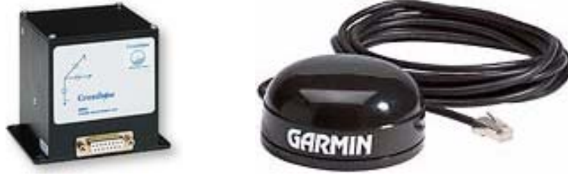
FIGURE 5 Sensors used in the INS. (left) The Crossbow DMU-HDX which is a solid state vertical gyro capable of measuring angular rates and accelerations on all three axes. It also has the capability of measuring the roll and pitch of the device too. (right) Garmin 16LVS OEM GPS which is both a receiver and antenna.
