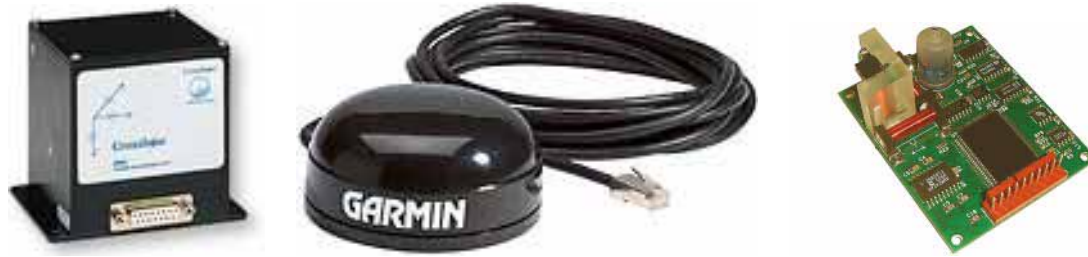
FIGURE 4. 5 Sensors used in the INS. (left) The Crossbow DMU-HDX which is a solid state vertical gyro capable of measuring angular rates and accelerations on all three axes. It also has the capability of measuring the roll and pitch of the device too. (middle) Garmin 16LVS OEM GPS which is both a receiver and antenna. (right) Precision Navigation TCM2-20 which is a digital compass capable of measuring direction and tilt information
